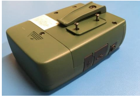
Figure 7. Loosen filter Cassette cover screws with a small Philips screwdriver
