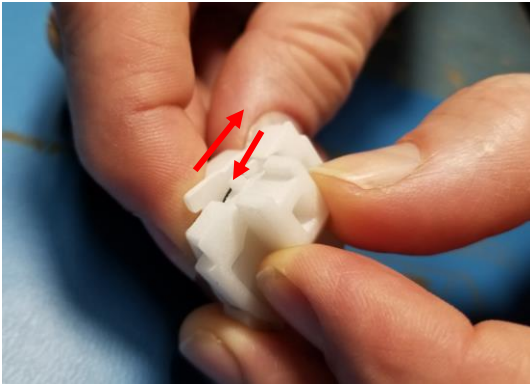
Figure 10. Twist the filter Cassette halves to unlock them, and then pull them apart
