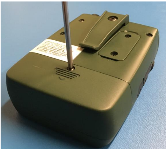
Figure 35. Loosening and removing Screw for Rear Battery Cover
