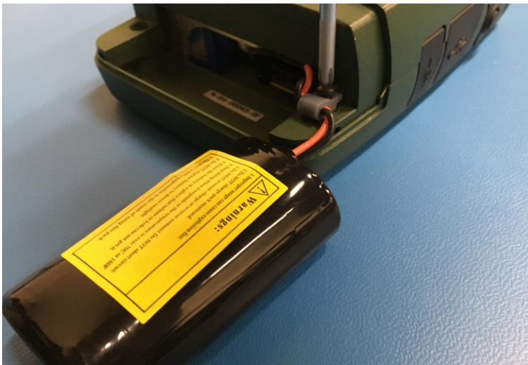
Figure 37. Removing Battery Cable Tie
