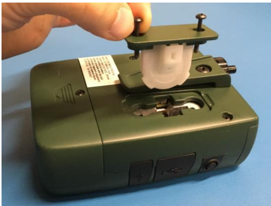
Figure 8. Extract filter Cassette by pulling up on the screws
