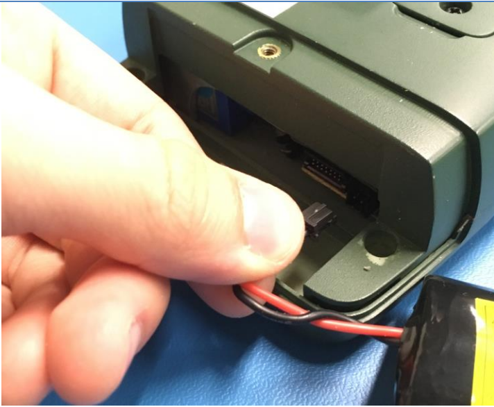
Figure 38. Disconnecting or re-connecting Battery
