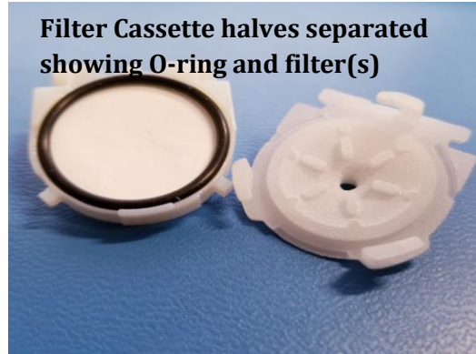
Figure 10. Twist the filter Cassette halves to unlock them, and then pull them apart
