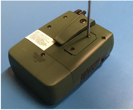
Figure 7. Loosen filter Cassette cover screws with a small Philips screwdriver
