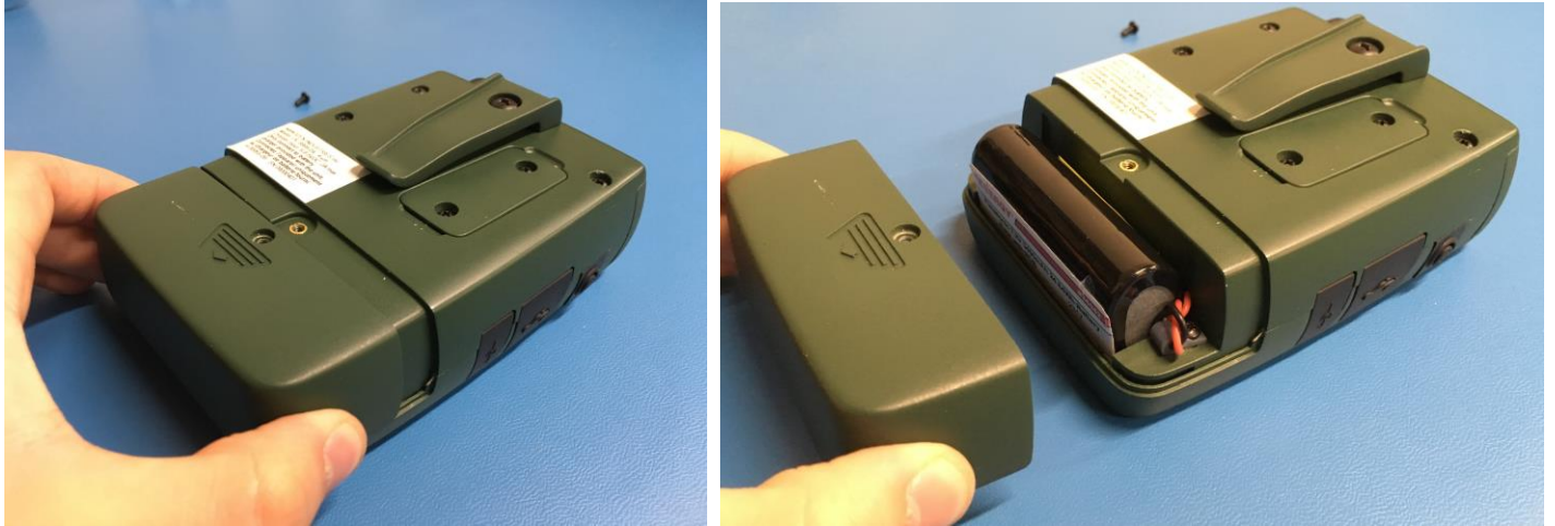
Figure 36. Sliding Off Rear battery cover
