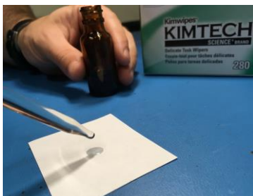
Figure 4. Use the Impactor Oil Applicator to apply one drop of oil to a fiber-free paper pad.
